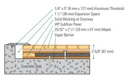
$\textbf{Slab Depression:}\ 25/32''\ (20\ \text{mm})\ \text{flooring} - 2^5/8''\ (67\ \text{mm}) \bullet 33/32''\ (26\ \text{mm})\ \text{flooring} - 2^7/8''\ (73\ \text{mm})$
